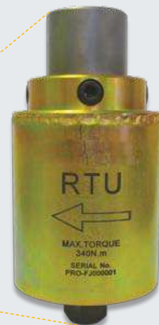
Modification of RTU for Track Bolt Tightening
