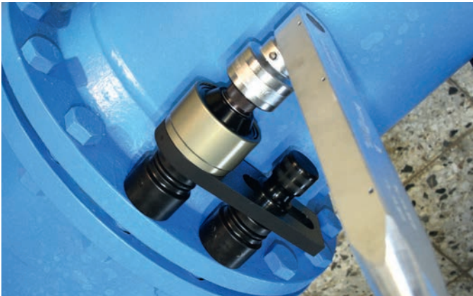
Popular for flange bolt connections: LKV-20/28L
